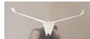
The tail flaps can be bent up slightly if the plane tends to dive. All changes should be made with small adjustments and then a test flight to analyze the change.
